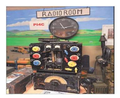
Their current operating activities use a WW2 RAF Wireless Operators table, complete with R1155 receiver and T1154 Transmitter.
