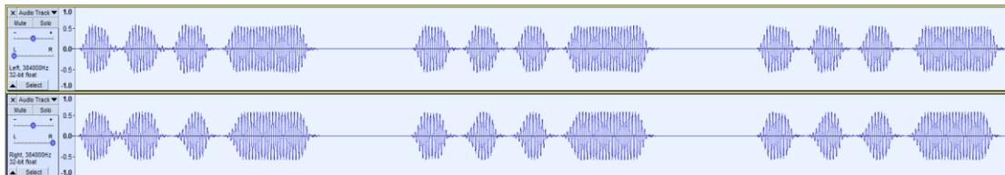
Figure 12: 60 WPM Rx Audio of the IC-7300 Tx signal: 2ms Rise time (top) and 8ms Rise Time (bottom)
