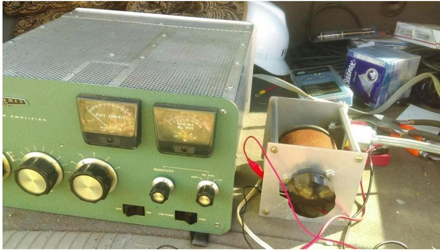
Since the amp hasn't been powered up for a while, I am bringing it slowly up to line voltage with a Variac. In the picture, I had crept it up to 56 VAC input. B+ was about 900 VDC.
