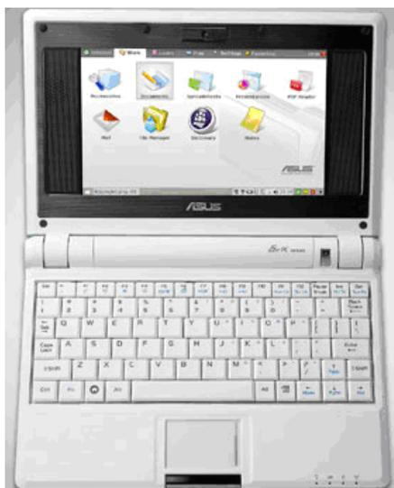
Shortly after its introduction, upon reviewing the specifications, I purchased an Eee model 4g for a hair under \$400, primarily for use during business trips. The unit measures less than 7 x 9 x 1 inch and weighs only two pounds. It has a 900 MHz CPU
