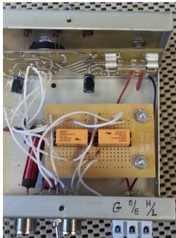
The relay board inside the Ameritron RCS-4 allows for the the 4-position rotary switch selections to be controlled by just two relays in the GH Everywhere system. Note the toggle switch. It allows the operator to return the control box back to normal manual operation. Another two relay positions change direction of the 4-square. 8 relays in the GH Everywhere remote module control the Array Solutions Six-Pak. It is impossible to have both K-3's connected to the same antenna at the same time.
