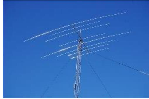
TX38 Triband Yagi Antenna
