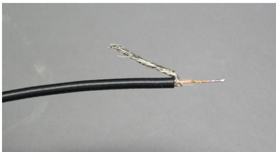
Figure 6. RG-174/U prepared for installing male TMP connector
