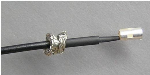
Figure 15. Inner heat-shrink in place.
