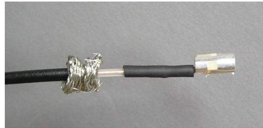
Figure 16. Outer heat-shrink in place.
