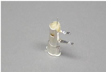
Figure 10. PWB-mount female connector.
