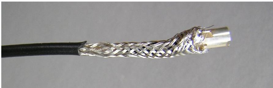
Figure 17. Braid soldered to connector shell.
