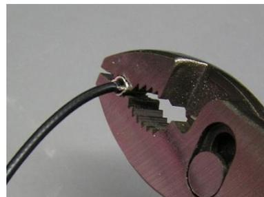
Figure 7. Using pliers to crimp the male TMP connector.
