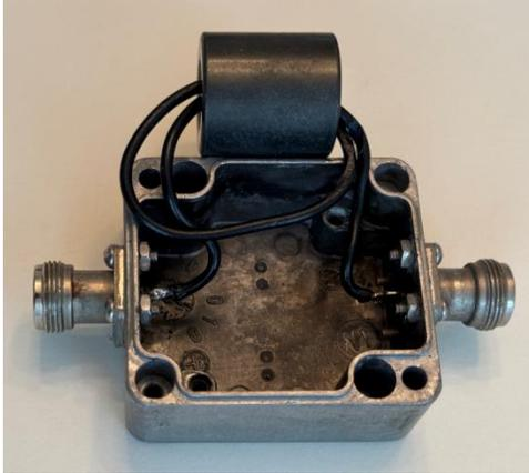
Figure 4 - A Simple Ferrite Test Set
