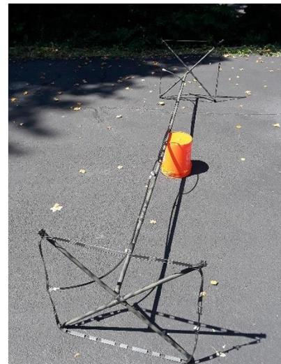
The elements that hold the 450-ohm ladder line are made of ½ inch PVC plastic plumbing pipe. The mast pole that separates the two elements is made of ¾ inch PVC plastic plumbing pipe. All connections are glued together with the correct type of PVC glue. Searching through Home Depot I found a 4 element [cross fitting](#).
