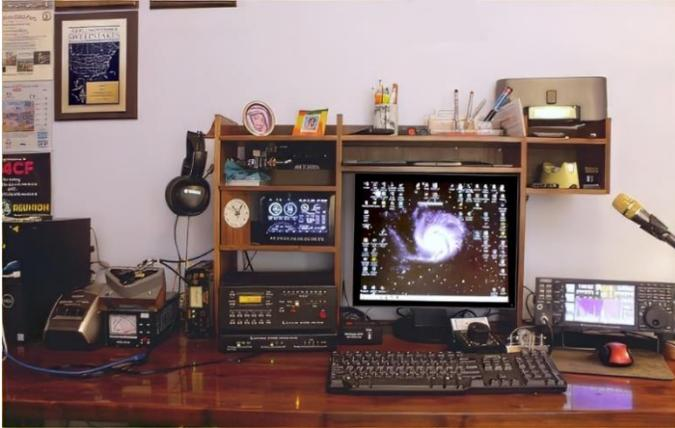
**Mike N4CF** It shares space with my home office on a 10-foot homemade walnut desk. On the right is an Elecraft K4D transceiver, and in the left hutch bay a KPA500 amp sits on a KAT500 tuner. To the left of the hutch are the main DC power supply, a dummy load, antenna switch, a label printer, and the office computer.
