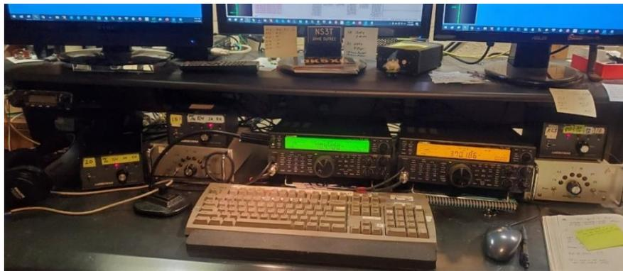
**Jamie NS3T** -I use a three monitor setup for contesting (you can only see the bottom of each monitor in the picture). I have a pair of TS-590SG rigs; I set the radios so that each one has a different color background. Each one has ICE-419A filters for SO2R operations. I also have remote antenna boxes for various bands on the shack table.
