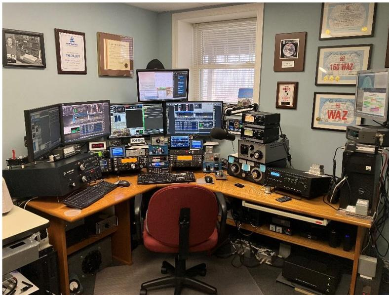
Mark K4SO Ergonomic layout with antenna selection centrally located. SixPak driven (both sides) by decoders on each K3. Easy to do the right parts.
