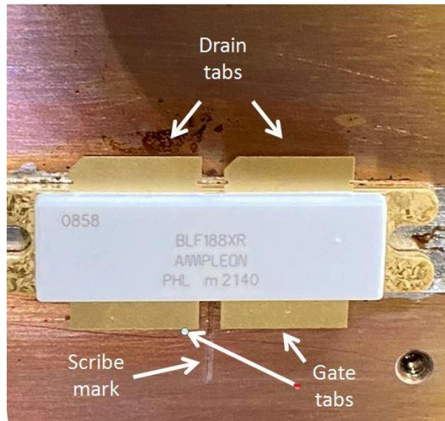
Figure 3 - BLF188XR on heat spreader
