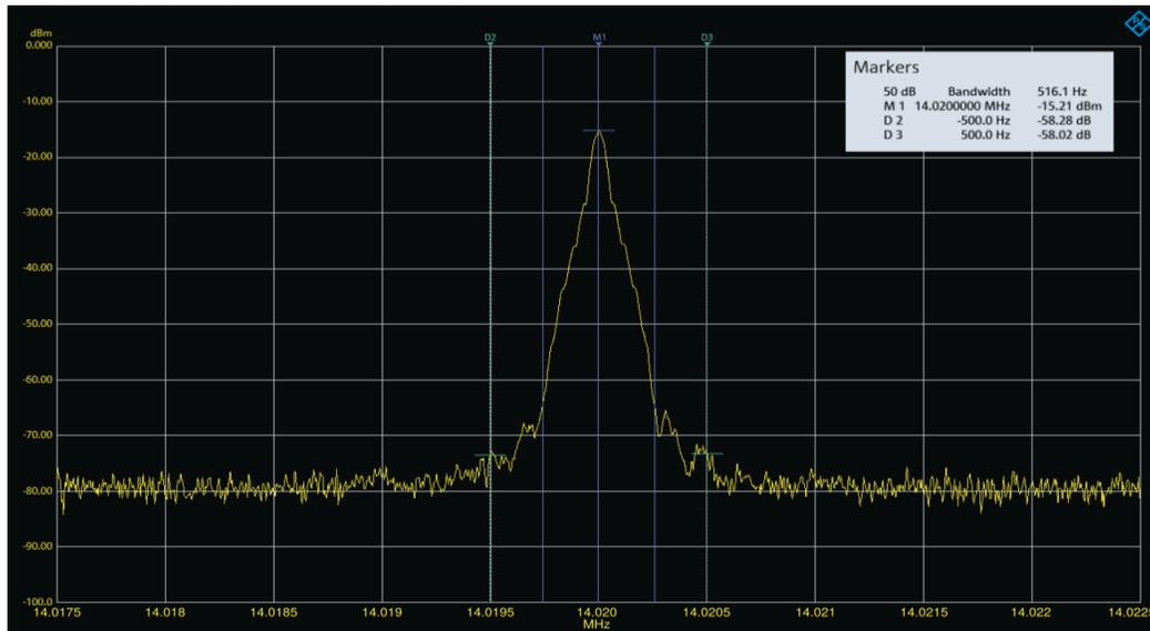
**Figure 4: K3 response in the frequency domain**
