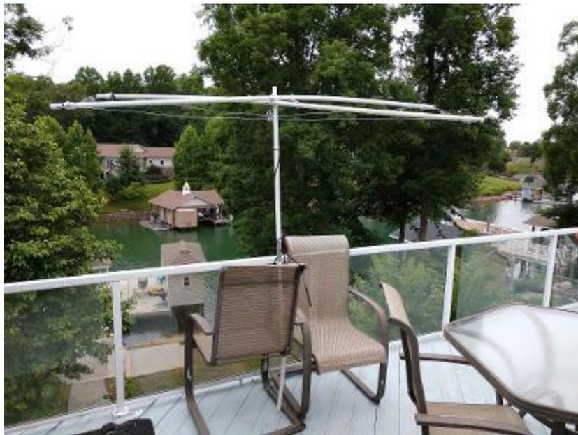
Here is my homebrew 6m Moxon constructed solely of PVC pipe, wire and hardware. Note the self-supporting tower. **Dana N6DW**
