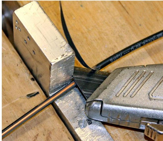
I clamped the jig in a vise, laid the wire in the notch, and laid the (new, sharp) blade in a utility knife on the wire, with the back of the blade bucked-up against the jig.
