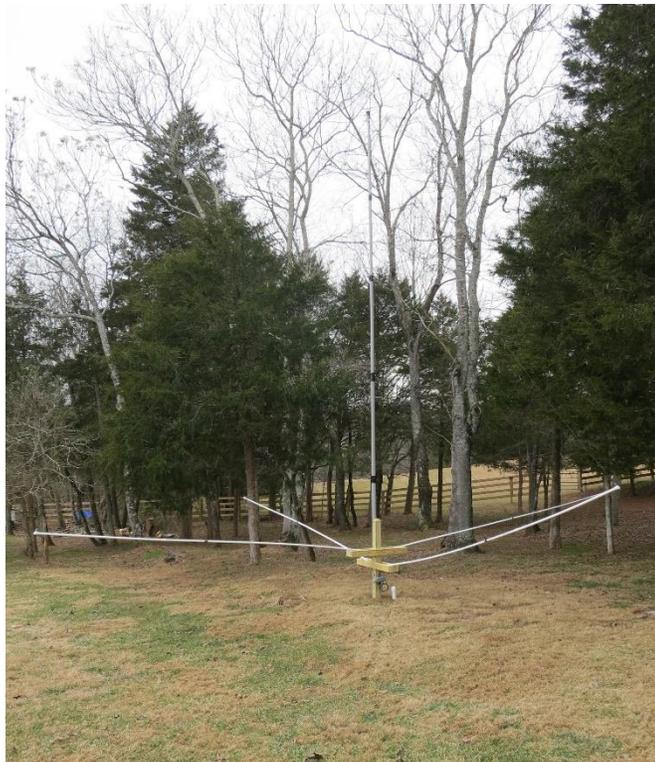
K9AY loop seen above, showing 28-foot mast and PVC spreaders. The spreaders fold up for grass cutting. With a center 4x4 post set in concrete, no guys or stakes are needed, and the design shown above has proven to be deer-resistant so far.
