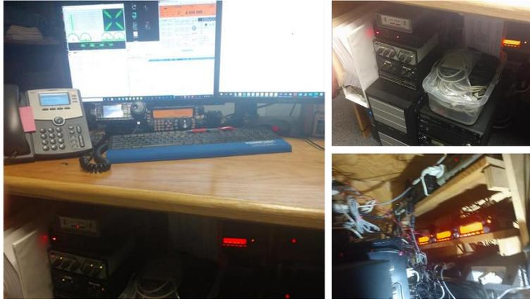
In its current configuration the primary station is a IC-7000 controlled by RemoteHams or ICOMS BA1 software, using a microHAM band decoder, Top Ten 6-way switch and multiple antennas onsite. It will be capable of 500W once I put the ICOM 2KL inline - I am only waiting on a way to remote switch power on and off. The second station is a TS-480HX which is on a 124ft doublet fed with 150ft of 600ohm ladder line to a MFJ-993 tuner. This station is primarily used on AFMARS.
