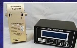
RF Power and SWR meter. Couplers for 3 kW, 10 kW or higher available for HF/6 m. VHF and UHF couplers for 1.5 kW. You can connect up to 5 couplers to the display to monitor RF power on different TX lines.
