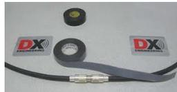
I use 3 layers of tape: Scotch 88 or 33+ first and last with 130c in between. The 130c is a rubber splicing tape we use at work. It gets applied sticky side out. This comes off fairly clean if you need to take it apart and reuse the connectors or cables. When you do that last wrap, don't tear the tape to finish. Cut it with a knife or scissors and finish the wrap without stretching to avoid it unwrapping later.
