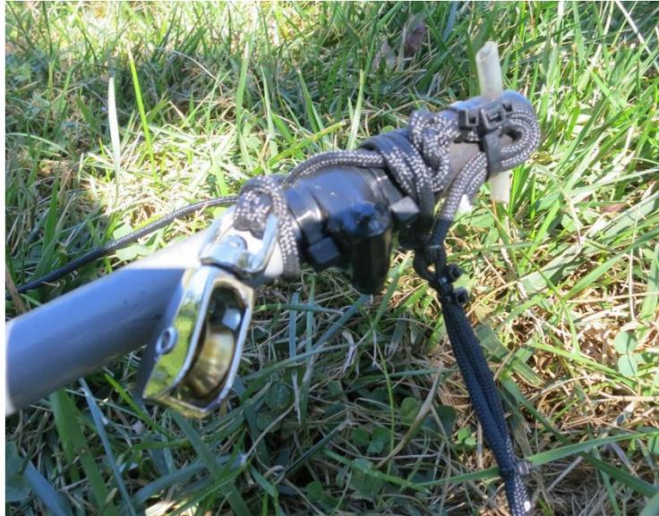
Figure 3. Top of Steppir pole showing two added guys and pulley.
