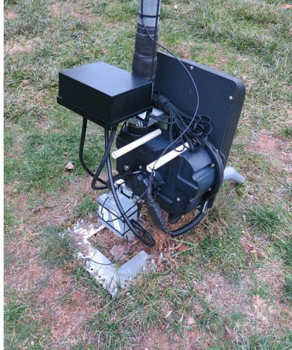
Figure 4. Steppir base with RCS-4 relay box, Balun Designs unun, and PVC standoffs .
