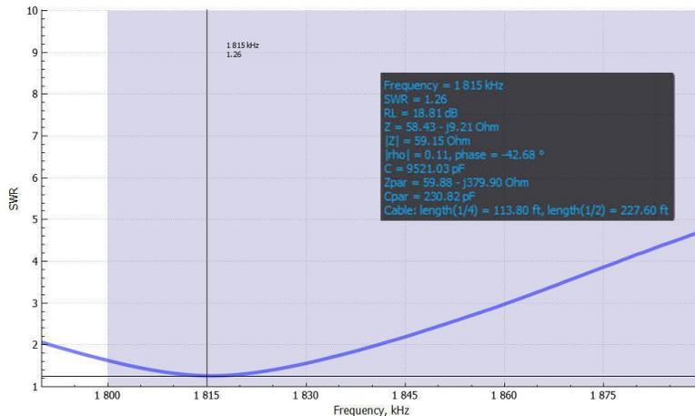
Figure 7. Inverted-L SWR.
