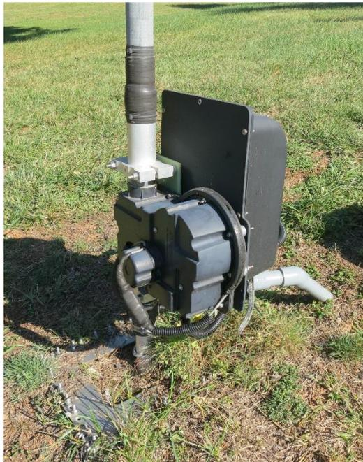
Figure 1. Steppir BigIR base as installed before 160 inverted-L was added.
