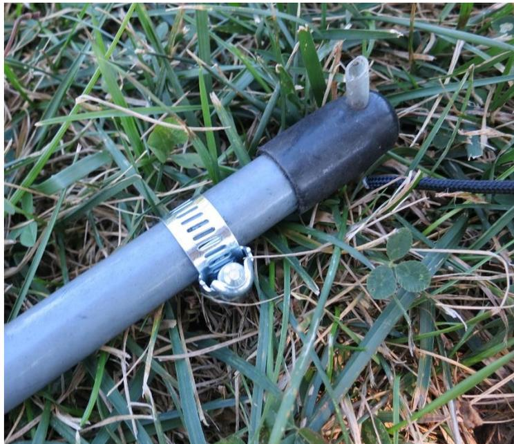
Figure 2. Clamp added to top of Steppir fiberglass pole.
