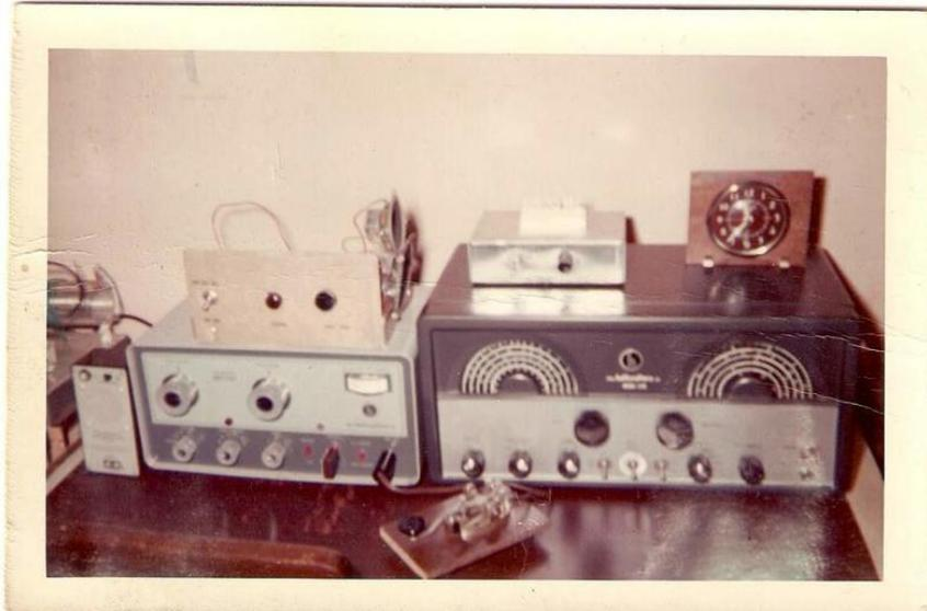
My H&H station- Hallicrafters and Homebrew. The cardboard front panel and cigar box chassis was an RF monitor for my monitor signal. The Bud chassis on top of the S-85 was an adjustable audio filter. The coil on turret standoffs way off to the left was my alligator clip adjusted antenna tuner. My favorite band was 15M and my first DX was F2RL. March 6<sup>th</sup> will mark my the 57th year of being QRV! - **Sid K3SX**
