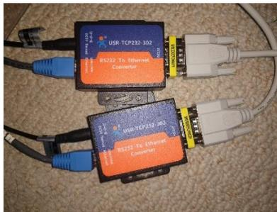
*Converters connected to Rotor-EZ and to my LAN switch.*
