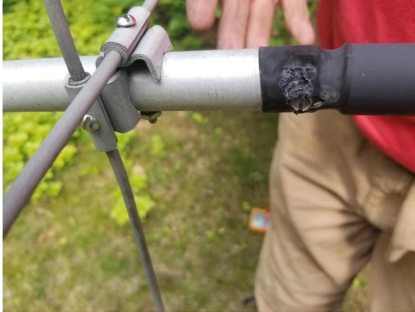
On the ground, we saw immediately what was wrong with the 40 m beam. It was what we had expected! At the end of one of the driven-element coils a stainless sheet metal screw that held the coil wire in place had loosened enough to cause a high-resistance joint. It was in plastic shrink wrap but apparently over time came loose. With high power there was arcing and scorching, quite evident once the antenna was on the ground. See the photo.
