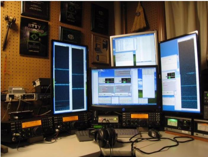
**Mark N2QT** - I keep changing looking for the best arrangement. These are for SO3R RTTY with waterfalls, so a bit more screen real estate needed than for cw/ssb. I use 2 or 3 pcs running a program called Synergy to allow sharing a single mouse and keyboard. WAE RTTY is the hardest on screen usage as QTCs take up a lot of room. Running multiple decode windows also takes up a lot.
