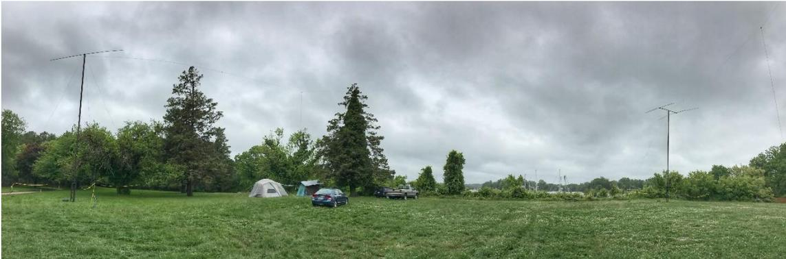
The antennas were all dipoles - 20, 17 and 15M were perched atop two 48 foot AB-577 military masts and the 80 and 40 meter dipoles were supported by 60 foot trees. Dipoles proved to be an ideal antenna choice because of Armed Forces Day activity was heavily concentrated east of the Mississippi, An eight man crew installed the all of the mast, antennas and tents in just four hours on Friday.
