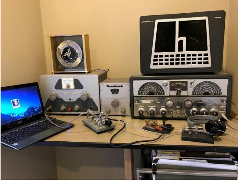
KN3DML 1958 novice station (sans VF-1). DX-40 and SX-100. (WN3R)
