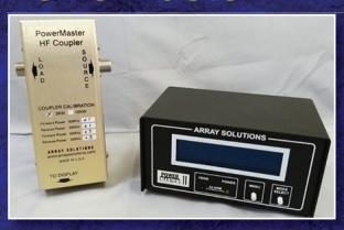
RF Power and SWR meter. Couplers for 3 kW, 10 kW or higher available for HF/6 m. VHF and UHF couplers for 1.5 kW. You can connect up to 5 couplers to the display to monitor RF power on different TX lines.
