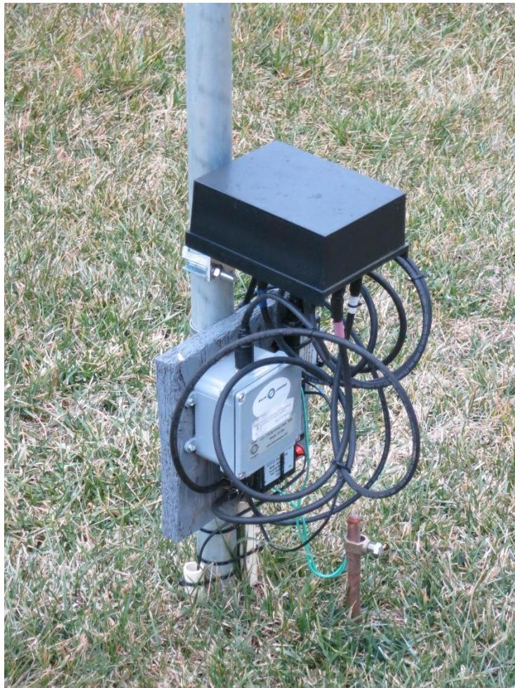
Beverage-on-ground hub, showing balun, feed and reflection transformers, and RCS-8V relay box.
