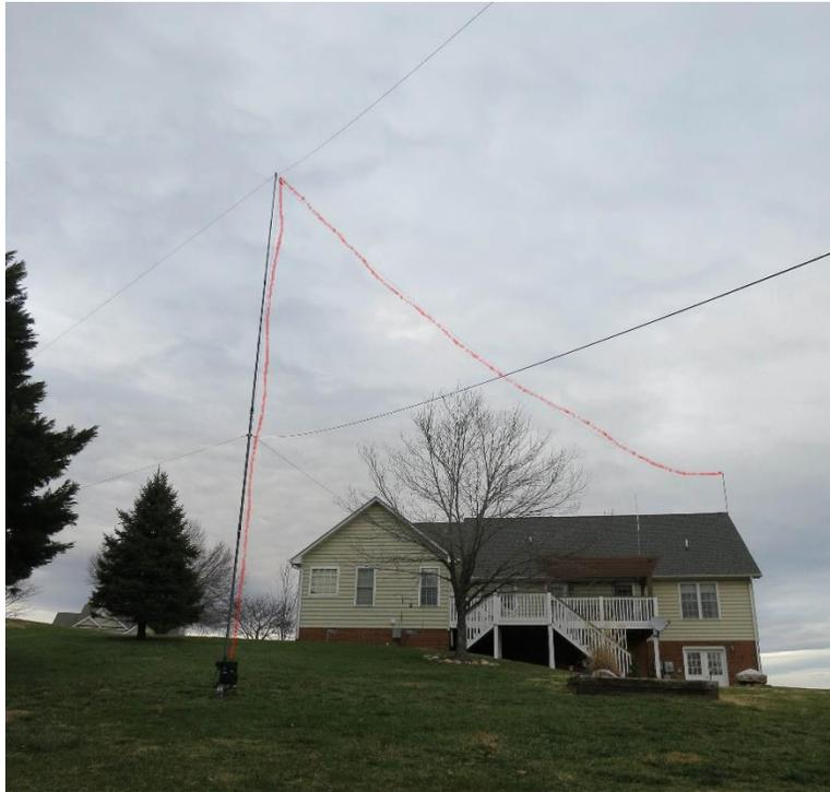
Figure 6. The Steppir BigIR, and the inverted-L, with inverted-L wire highlighted in red.
