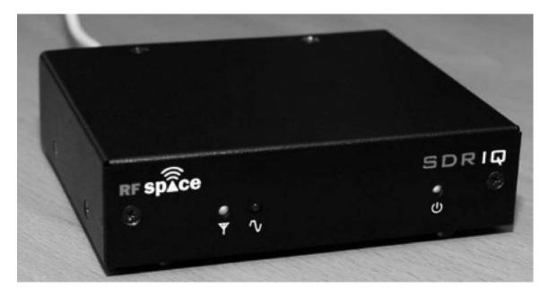
For that you get a very competent general coverage receiver, with up to 190 KHz bandwidth from 500 Hz to 30 MHz, in a very compact package. The SDR-IQ does not need a sound card. Instead, a single USB connection handles data, control, and power for the receiver. The SDR-IQ package includes very sophisticated spectrum analyzer, called *Spectravue*. One argument for this option is the other things you can do with the unit when you're not contesting, from VLF to SWLing.
