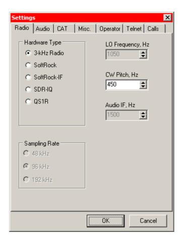
Start with the Radio tab. Select 3-KHz radio. Then set the CW pitch you like – that will determine the pitch of CW you hear in the speaker (if you have the speaker on) and the accuracy of the frequency readout, so set it to your accustomed pitch. Now click on the Audio tab.
