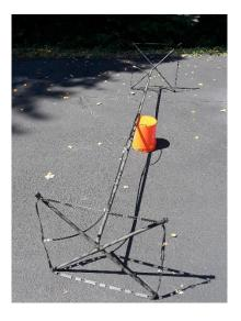
The elements that hold the 450-ohm ladder line are made of ½ inch PVC plastic plumbing pipe. The mast pole that separates the two elements is made of 3/4 inch PVC plastic plumbing pipe. All connections are glued together with the correct type of PVC glue. Searching through Home Depot I found a 4 element cross fitting.
