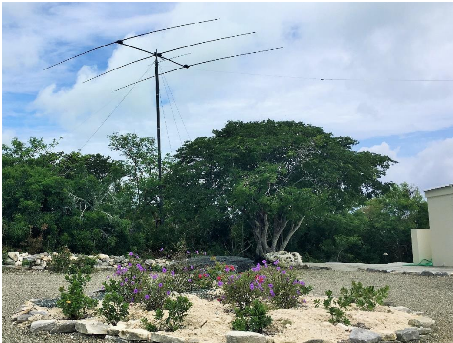
Mast with SteppIR and Inverted V
