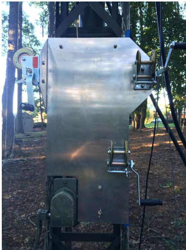
Bare panel with the winches attached before we added the lines and carabiners.
