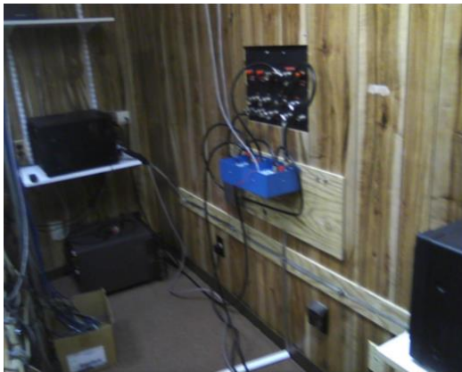
Two Stack Matches will be used for IARU, two more will be installed for SO2R.
