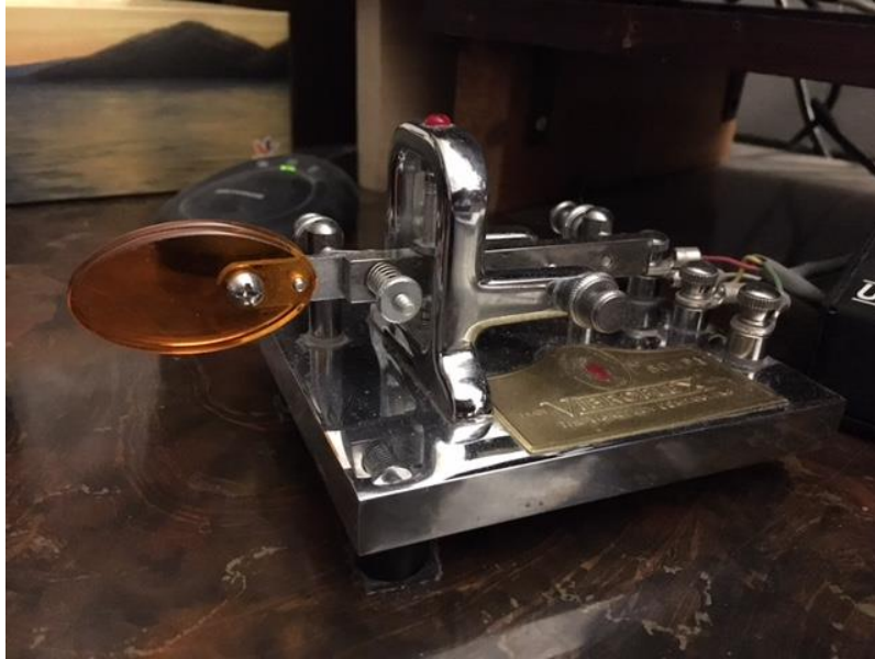
Sid K3SX - Here is my single lever Vibroplex paddle with custom finger pieces from 2B Radio Parts LLC . They are light weight but do not flex.
